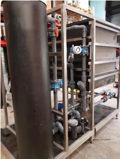
The small ultrafiltration system continues to be assembled by our supplier in the Netherlands. The latest photograph provided (at left) shows the frame and the filtrate tank installed together with two pumps. The control panel and the filtration modules will be installed in February with shipment to Qponics expected at the end of that month. A large specialised algae centrifuge is expected to be purchased and installed in February.
